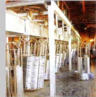
热镀锌铁丝高锌层生产线 (BWG6-BWG16) The production line of hot dipped galvanized wire for thick coated zinc
